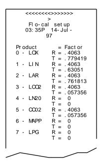
Note: Each SP1200 is factory calibrated for products and engineering units of total as specified by user.
